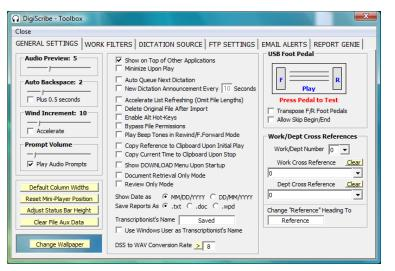
**Wind Increment:** Select the number of seconds to Rewind or Fast Forward for each second the Rewind or Fast Forward foot pedal is pressed. Adjust from 1 to 60 seconds. Check **Accelerate** to accelerate the wind increment as you continue to press the pedal.
